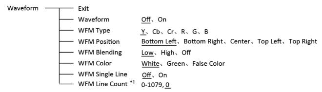
\*1: Only the "WFM Single Line" is set to "ON", the "WFM Line Count" can be adjusted. "WFM Single Line" is to display the selected line waveform of "WFM Line Count"
