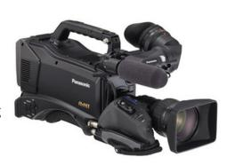
1/3" sensors are generally used in handheld cameras. There are some 1/3" sensor shoulder-mount cameras, but by and large the smaller sensor is typically used in handheld models. These cameras also generally have fixed (non-interchangeable)
