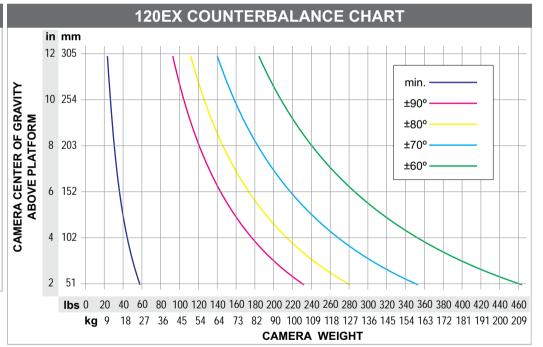
Now, with the use of EX-technology OConnor can offer the features it has become famous for while offering an additional benefit: extended capacity. With a new counterbalance mechanism at the heart of the EX-technology, the 120EX can be boosted into EX-mode to achieve a whole new realm of counterbalance.
