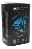
Capacity: Max Output Voltage Nominal Voltage: Max Draw: Power Outputs: End Voltage: Additional Features: Protection: Ambient Temperature: Dimensions: Weight: 179Wh 16.8V 14.8V 12A (1) 80W D-Tap 11.2V 4-LED Power Indicator Over-charge, over-discharge, over-current 32°F ~ 104°F (Charge), -4°F ~ 113°F (Discharge), -4°F ~ 113°F (Storage) 3.82(W) x 5.75(H) x2.32(D) inches 2.31 lbs
