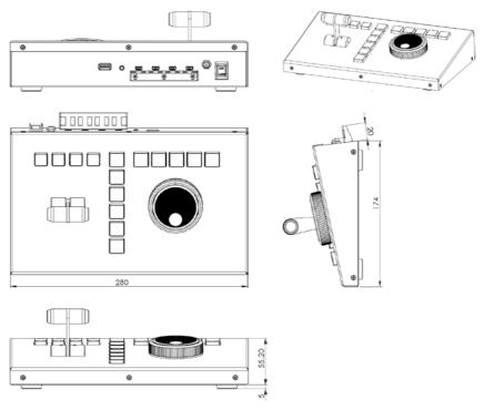
All measurements in millimeters (mm)
