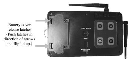
Insert six AA batteries into the battery sled, in the positions shown inside the sled, and install the sled in the battery compartment as shown below. An HME BAT850 Rechargeable NiMH Battery may be used instead.
