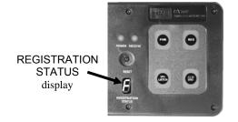
Clear all current registrations from the base station by pressing the CLR/BND button and the RESET button at the same time.
