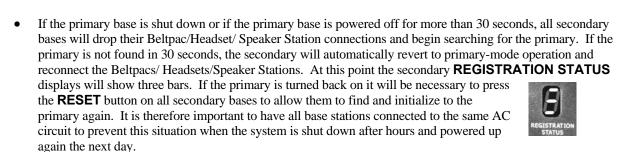
**NOTE:** You cannot register Beltpacs/Headsets/Speaker Stations to a base that is set to primary mode, and then switch the base mode to secondary for initialization. Once in secondary mode, the base cannot recognize the Beltpacs/Headsets/Speaker Stations registered during primary operation. For secondary bases, the Beltpacs/Headsets/Speaker Stations must always be registered after secondary base initialization, with the primary base remaining active and the secondary base displaying one bar.
