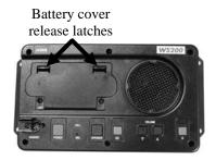
• Insert six AA batteries into the battery sled, in the positions shown inside the sled, and install the sled in the battery compartment.
