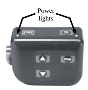
• **Power Off** — Press and hold the **PWR** button for approximately 2 seconds. A voice message in the earpiece will say "Power off," and the green power light will go off.
