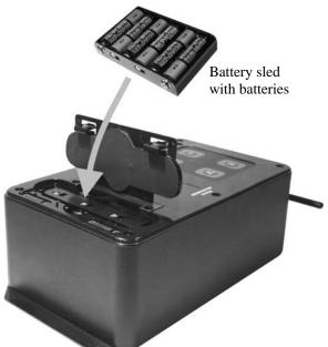
Close the battery compartment by pressing its cover down until both latches snap in place. **NOTE:** Pressing down on the cover next to both of the latches at the same time will assure its proper closing.
