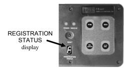
Clear all current registrations by pressing the CLR/BND button and the RESET button at the same time. Continue holding the CLR/BND button after you release the RESET button, until the clear code "C" (lower case) appears on the REGISTRATION STATUS display.
