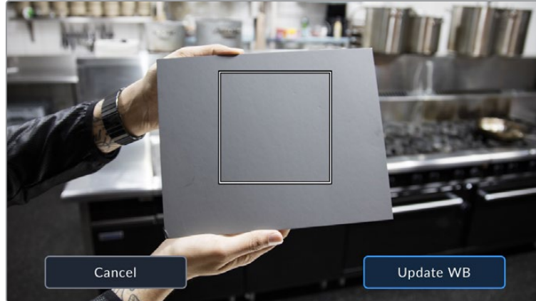
Tapping the 'AWB' icon in the white balance menu will bring up the auto white balance screen. Use this with a white or neutral gray surface to automatically set a neutral white balance
