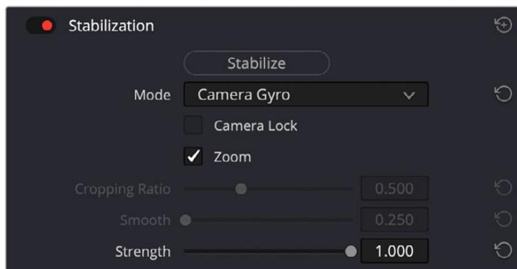
In the inspector window select 'camera gyro' to stabilize the clip using gyro data
