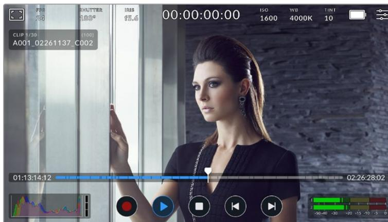
A timeline of segments represents all the recorded clips and each segment represents an individual clip. The current clip name and number is shown at the top left of the display and the total number of clips on the card or drive is shown in brackets.
