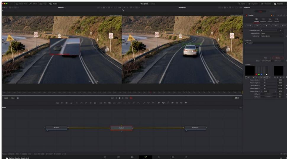
Tracking options in the inspector panel include track reverse from last frame or current frame, stop track or track forward from current frame or first frame.
