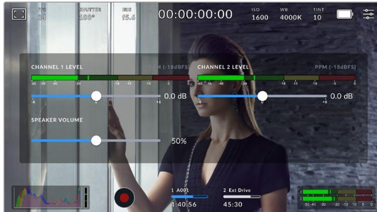
Tap the audio meters on the LCD touchscreen to easily access volume and headset or speaker settings
