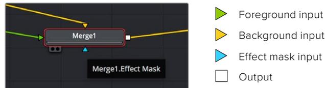
Multiple outputs on nodes means a single node can connect to many different nodes in your composition, so you don't have to duplicate clips as you would in layer based software. Arrows on the line between connected nodes are a great visual indicator to show you which direction the image data is flowing.
