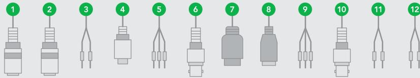
1. Audio Input • 2. Audio Output • 3. RS422 Connector (Combine with 11) • 4. Upgrade Interface • 5. Alarm Input
