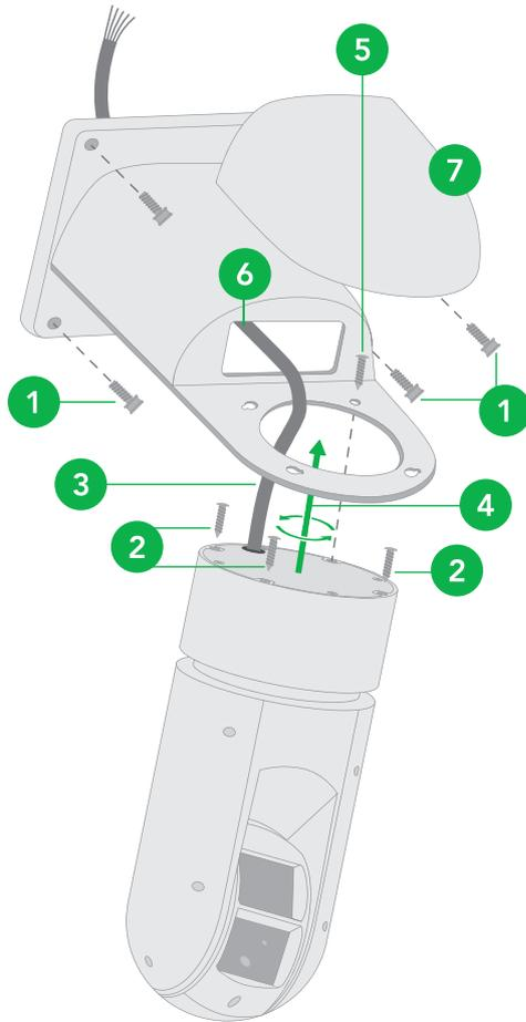
1. Open the bracket cover, mount it onto the wall or pole (use pole adaptor).
