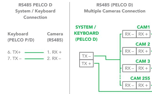
Connect the Camera's RS485+ and RS485- to RS485/TX+ and RS485/TX- on the control system/keyboard. The identity of the control system or equipment may be different; the corresponding relationship is as follows:
