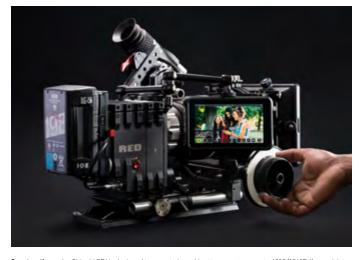
Construction note: Shinobi SDI is designed to operate in ambient temperatures up to 40°C/104°F. If you wish to extend the temperature of operation in high temperature conditions, set the TFT brightness to a minimum.
