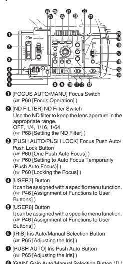
[GAIN] Gain Auto/Manual Selection Button / [L/ M/H] Sensitivity Selection Switch (INP P66 [Setting the Gain]) [WHT BAL] White Balance Auto/Manual Selection Button / [B/A/PRESET] Selection Switch
